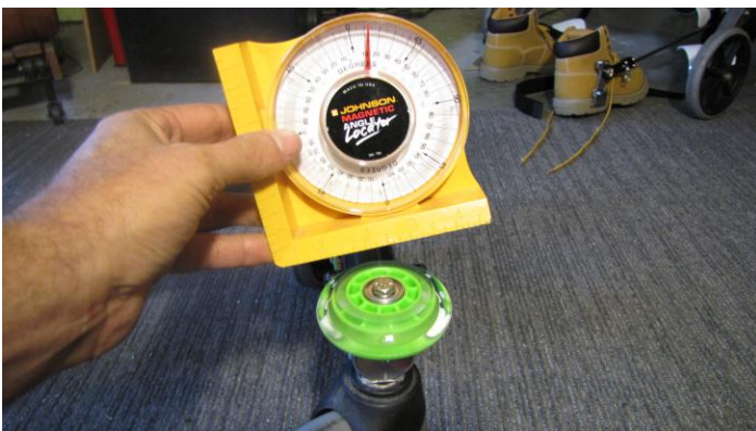
Step 5: Level the wheel. Level equals less wall marking. (You can use a level as shown or just use your eye to do it.)
