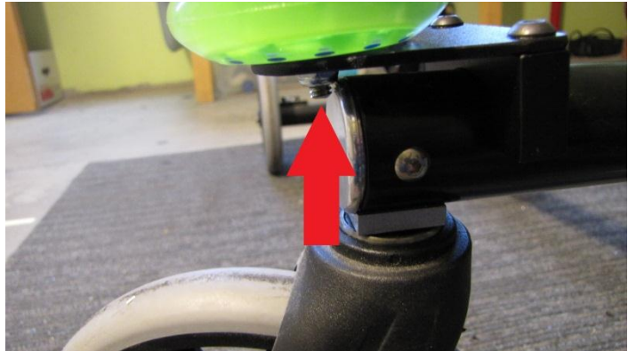
Step 2: place wheel/clamp with bolt past tube.
